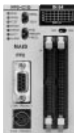
FP2 CPU unit with 64-point input FP2-C1D
